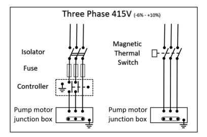
Check rotation of the motor (three-phase motor). The motor fan should be spinning in a clockwise rotation. If the fan rotation is incorrect, isolate power to the pump and exchange the two supply wires.
