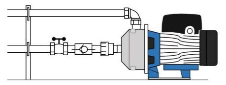
Mount the pump on a firm base in a dry, free draining area
